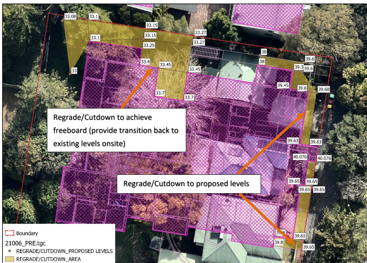
Figure 8.3.1: Site Regrading in TUFLOW model
