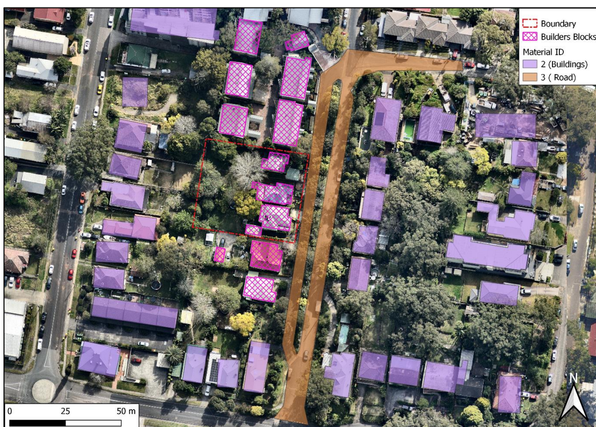
Figure 8.4: Material ID Map in TUFLOW model
