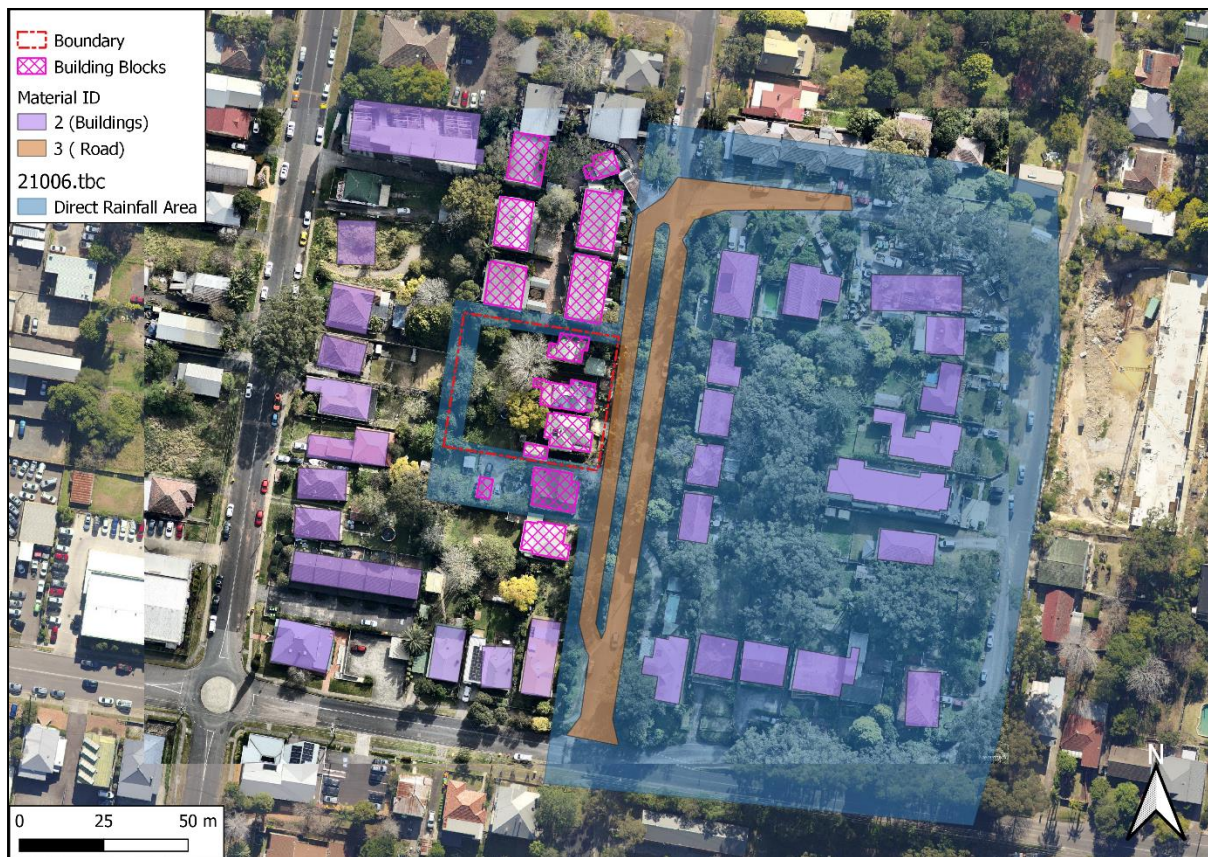
Figure 7.1.1: Direct Rainfall Catchment
